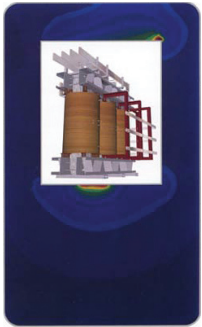
Image 2: Shows a graphical representation of the intensity level of the electromagnetic fields outside of the enclosure of a shielded transformer. Due to magnetic shielding of the enclosure most of the field emission is contained within the transformer enclosure.
